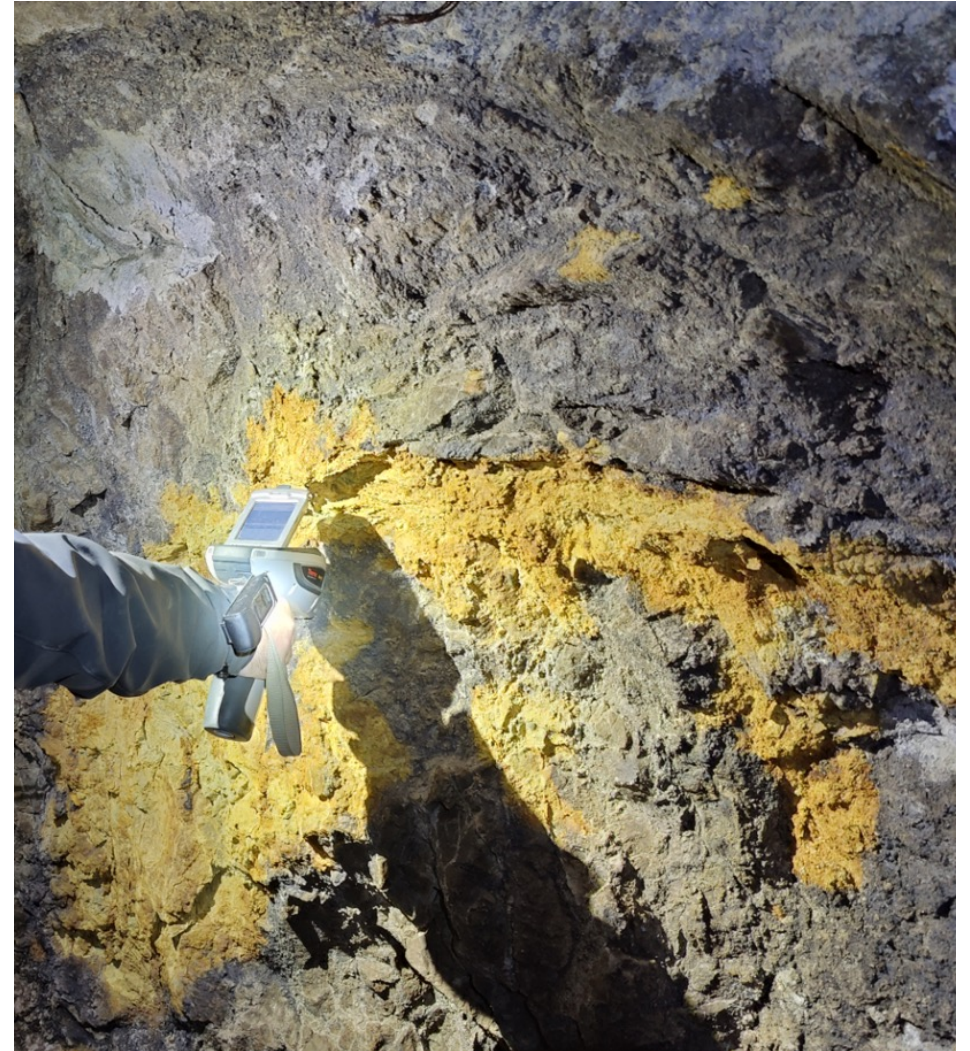
Altered and pervasively Zn-Pb-Ag-mineralized carbonate (gray) in G2, exhibiting partial oxidation of accompanying Fe-sulphide (ocre).
