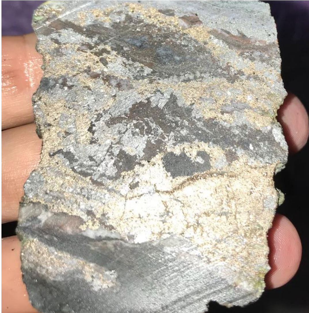
Left: Stringers of silvery-golden Co-Ni mineralization in low grade metamorphic sediments (gray) from the waste dump of G7.
